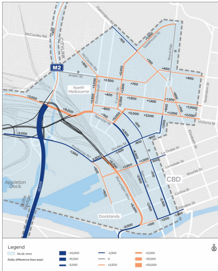
Figure 25-6 Difference in daily traffic volumes - West Melbourne and North Melbourne – 2031 project case vs 2031 no project case
